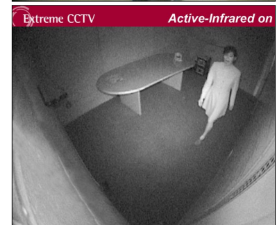
Above: The EX36MNX uses active-infrared to “invisiblely” illuminate a room, an important capability in sleep research.
